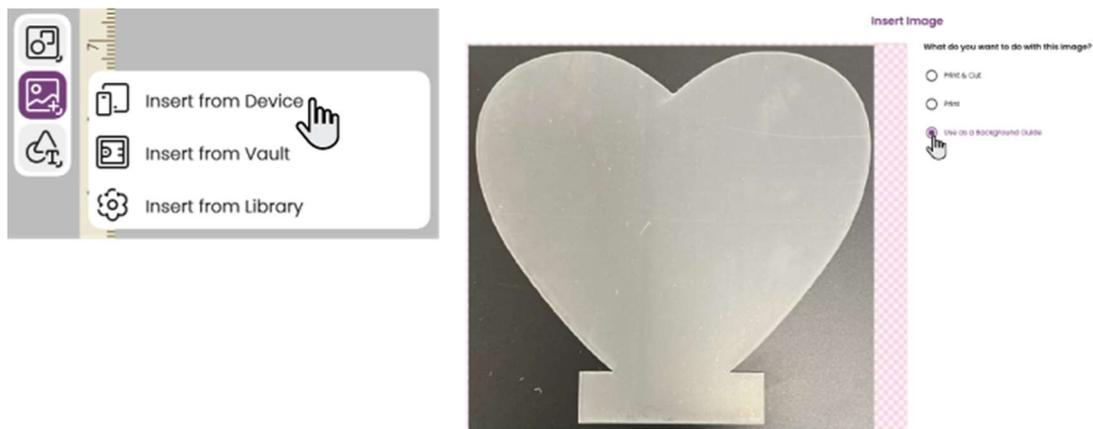
3. Measure your acrylic blank. Resize the image so that it is the same size as it is in real life. Move the image so that it is not on the edge of the mat, using the lines as a guide. Lock the guide layer to prevent it from accidentally being moved. Go to Object – Lock. You can also lock an object by using the Ctrl+L shortcut on the keyboard or by clicking the lock symbol in the filmstrip.
